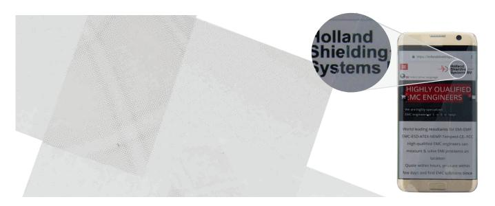
This transparent conductive Metal Mesh PET film is optical PET film deposited with copper grid and protected with a nickel layer. This film conducts better than our best 9900 series Transparent shielding foil and is only a fraction less transparent. This film has a conductive layer with a very fine etched mesh that is one with the transparent carrier.
